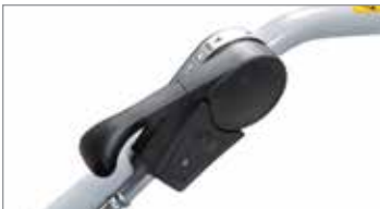
Handlebar-mounted PTO control.
