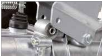
Handlebar mounted on vibration dampers.
