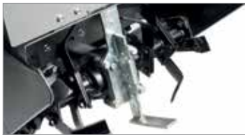
Rotor depth adjustment enables operation on all types of terrain.
