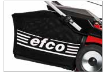
The large canvas grass catcher with 80-litre capacity ensures fewer emptying stops.
