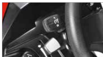
The cruise control function allows you to set a constant ground speed and thereby get the job done more efficiently.
