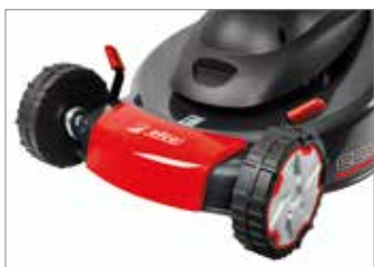
Independent cutting height adjustment on each wheel.
