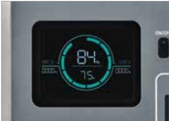
The display shows various information such as remaining charge status, instantaneous load, or input charging power.
