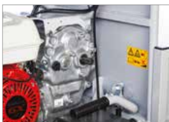
Independent 2100 rpm PTO.
