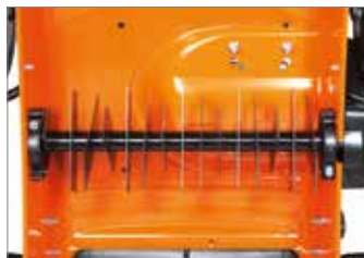
Rotor comprising 15 fixed blades.
