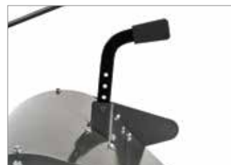
50 cm rotor with depth adjuster.
