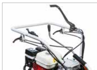
Steering with independently controlled release and brakes.
