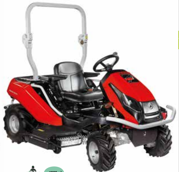
110 cm cutting deck with 3 rotors and 6 mulching blades for finely chopping all types of grass and shrubs (TONKAWA 110).
